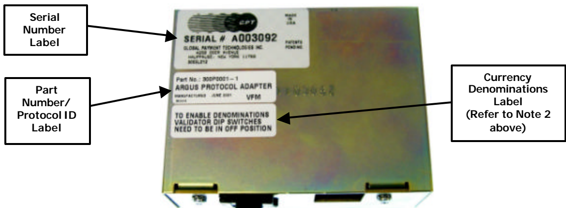
Figure 2. Protocol Adapter Assembly – Label Identification
