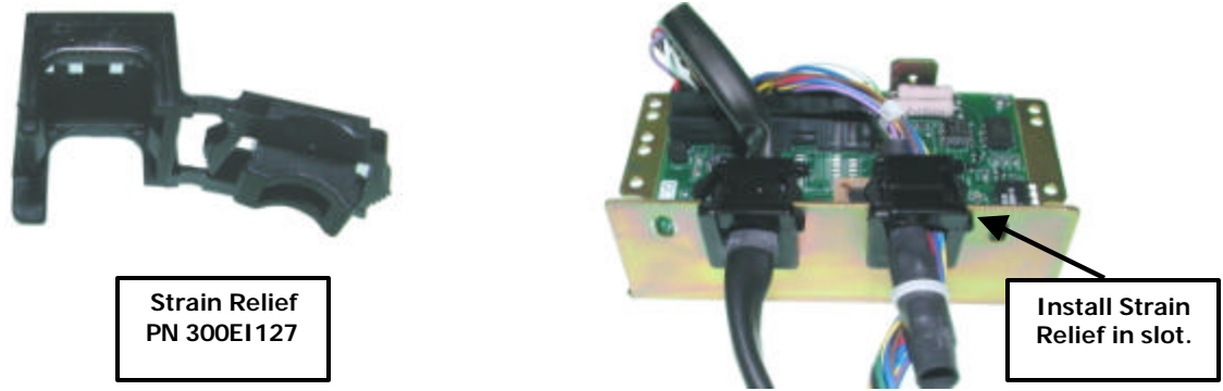
Figure 7. Installation of Strain Relief
